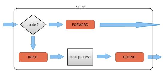
Figure 7. Firewall Chains: Input, Output and Forward
